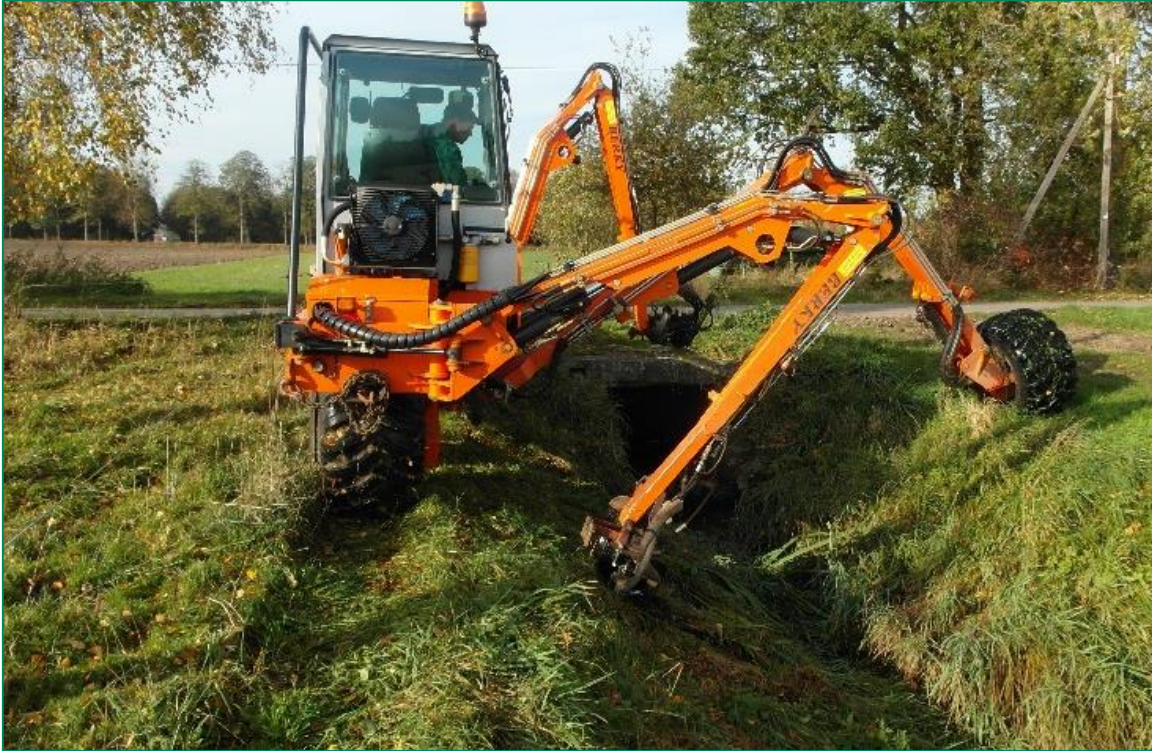
Extended stabilizer mowing bar
