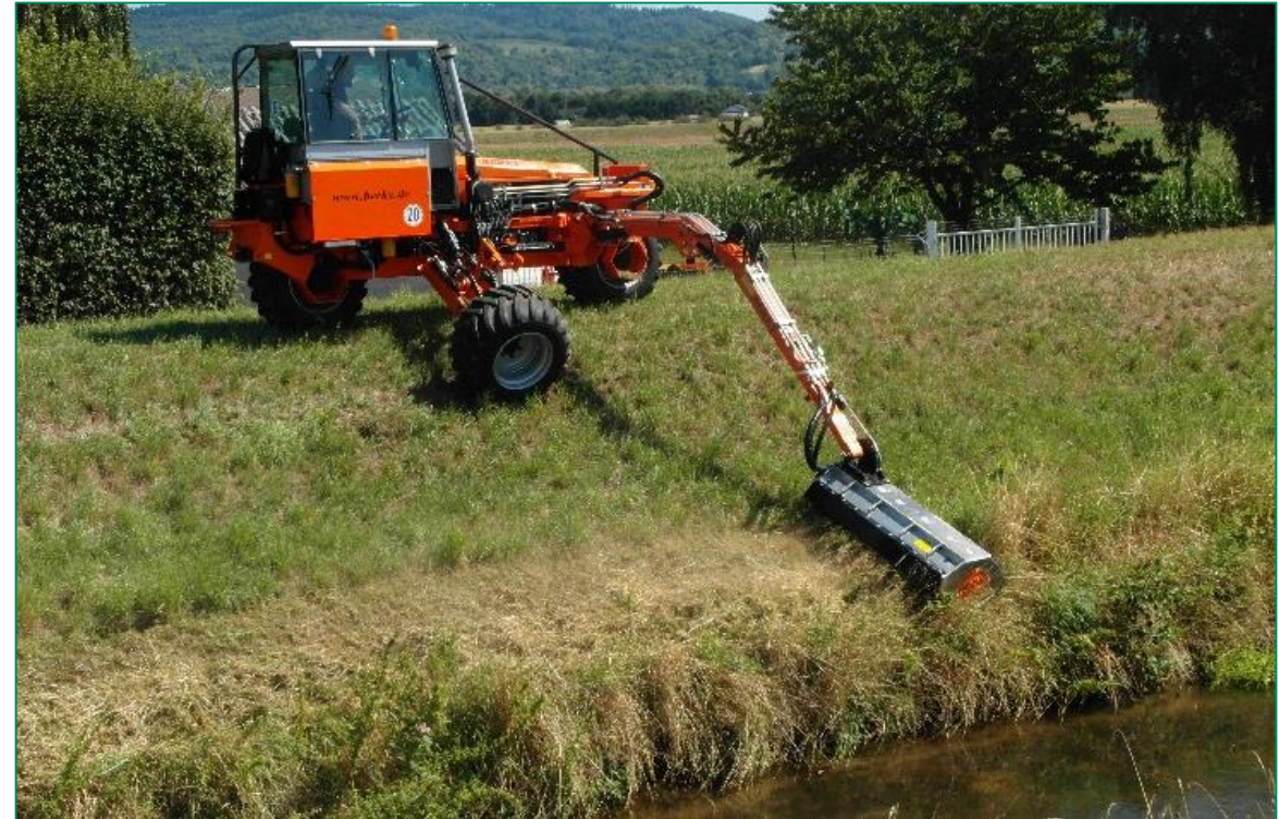
Rotary chopper with standard stabilizer berm cutting
