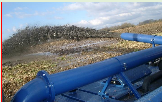
⚙ SIDE CASTING SYSTEM OF SPOILS & MUD ON LAKE SHORES, RIVERS & CANALS
