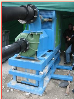
⚙ BOOSTER PUMP STATIONES FOR EXTRA LONG DISTANCE PUMPING
