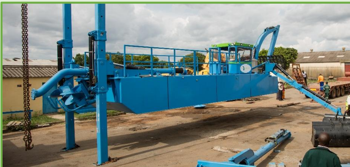
FOLDING SPUD ANCHORS. DUAL USE: SELF-LOADING & IN LAKE ANCHORING
