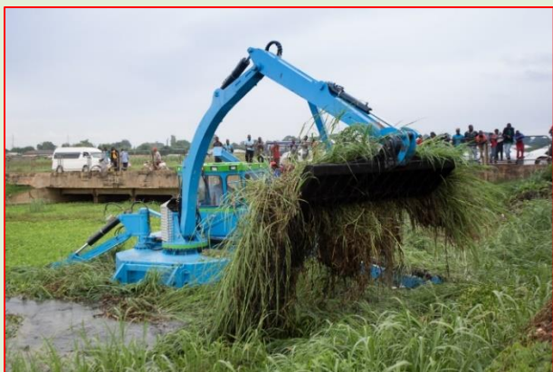
REVERSIBLE RAKE FOR WEED & ROOT REMOVAL & SHORE LINE MAINTENANCE
