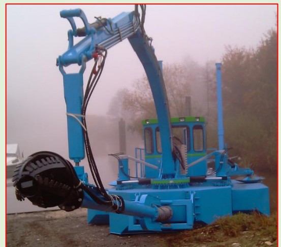
⚙ "SWINGING-LADDER" WITH A HUNGRY FOR WORK CUTTER DREDGE HEAD
