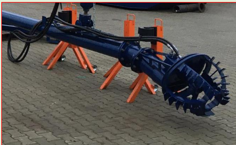
⚙ "SWINGING-LADDER" WITH A HUNGRY FOR WORK CUTTER DREDGE HEAD
