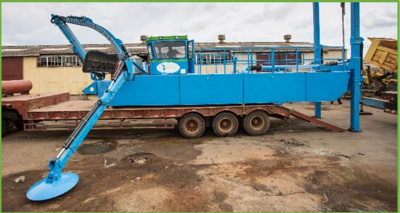
FOUR “LEGS” WORKING TOGETHER FOR SELF-LOADING ONTO TRUCK
