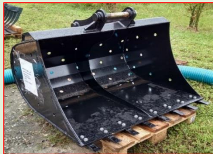
⚙️ EXCAVATING BUCKETS: CLOSED, PERFORATED & EXTRA WIDE
