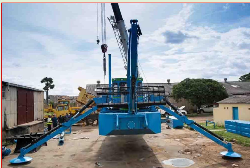
BOW STABILIZERS DOING THE "SPLITS" & LIFT
