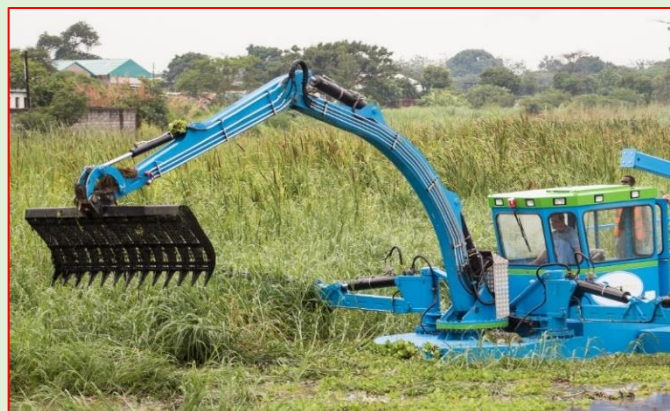
REVERSIBLE RAKE FOR WEED & ROOT REMOVAL & SHORE LINE MAINTENANCE
