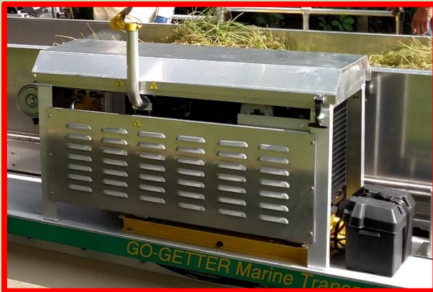
Diesel Engine-Hydraulic Power Unit ⚙️ Console w. Remote Controls
